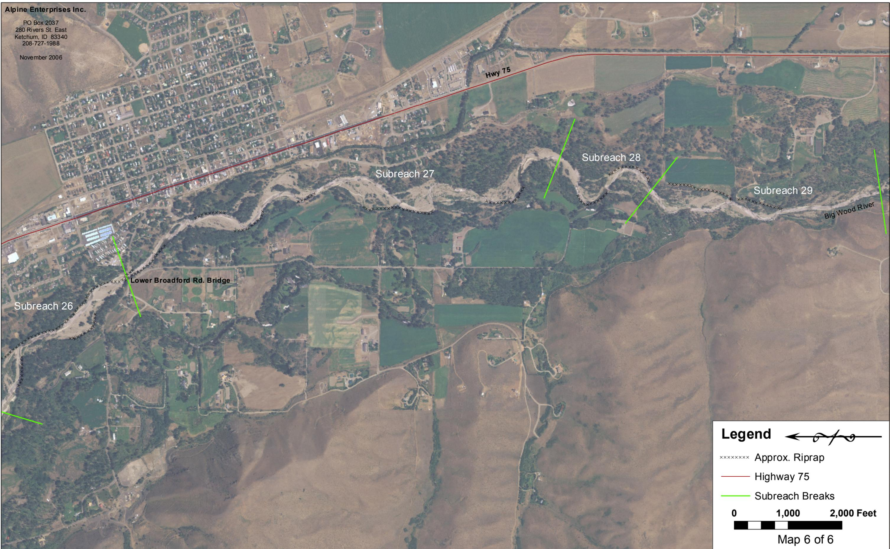
Figure 5 (Sheet 6 of 6). Results of the preliminary bank hardening survey for the Big Wood River within the study reach.
