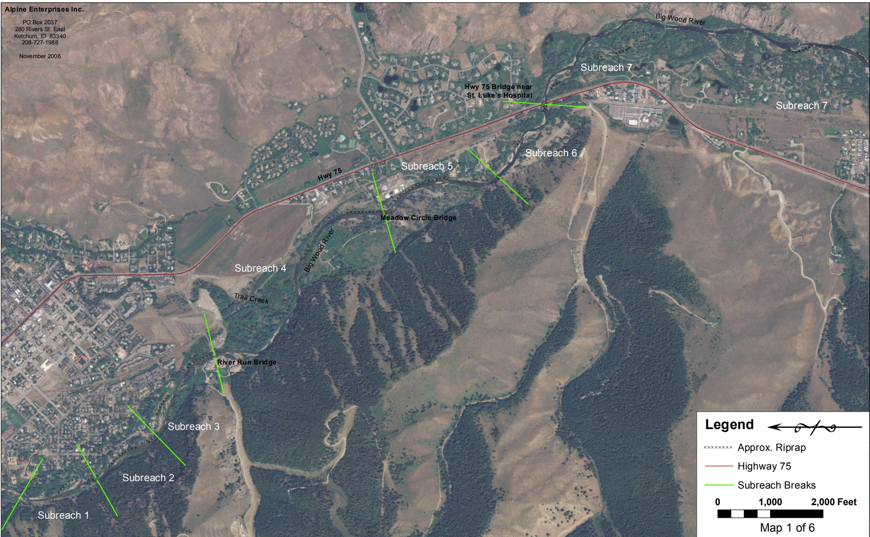
Figure 5 (Sheet 1 of 6). Results of the preliminary bank hardening survey for the Big Wood River within the study reach.
