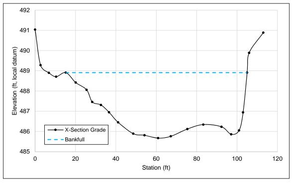
Figure 93. Typical riffle cross section of the main channel in the Colorado Gulch Reach.
