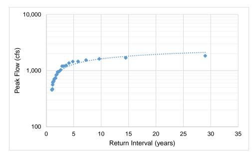
Figure 1. Peak flow recurrence interval at the USGS Big Wood River gauge near Ketchum (#13135500).
