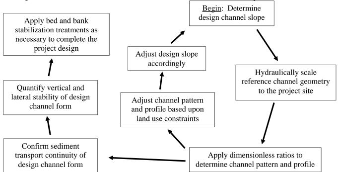
Figure 110. Generalized design process diagram.
