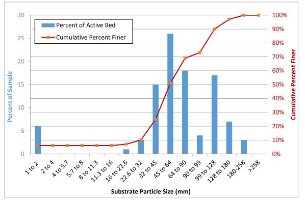
Figure 109. Surface particle size class distribution in the Glendale Reach.
