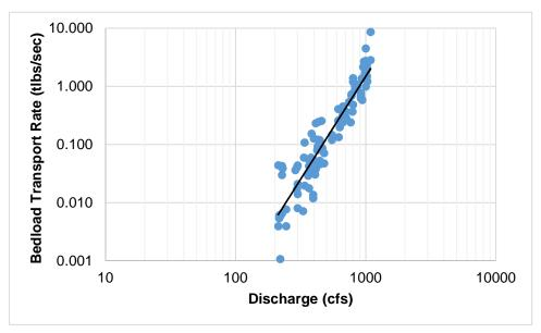
Figure 4. Bedload sediment transport rating curve, North Fork Campground on the Big Wood River.
