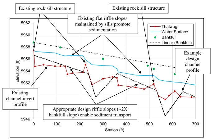
Figure 132. Existing and example design channel profile proximate to sills in the Training Channel reach.
