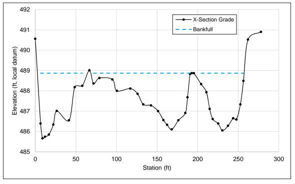
Figure 80. Typical riffle cross section across multiple channels in Downstream of Deer Creek Reach.
