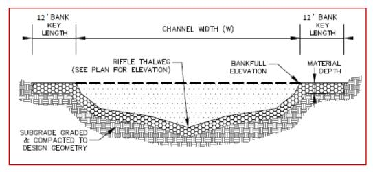
Figure 129. Section view of typical hardened riffle treatment design.
