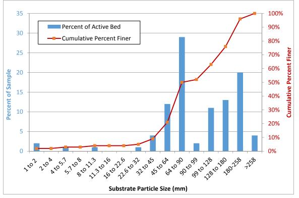
Figure 73. Surface particle size class distribution in the Downstream of East Fork
