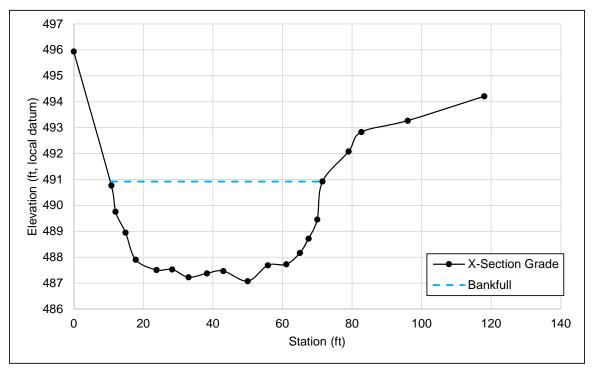
Figure 27. Typical riffle cross section at Fox Creek Reference Reach.
