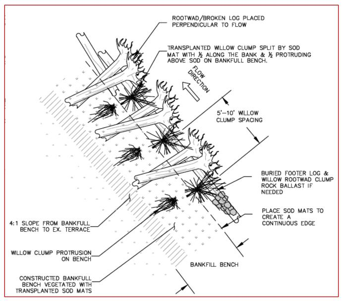
Figure 117. Plan view of typical wood revetment bank stabilization treatment.
