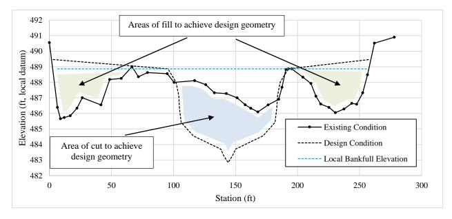
Figure 113. Example existing and design channel geometry from Big Wood River downstream of Deer Creek Site.
