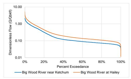
Figure 3. Dimensionless flow duration curves developed from USGS Big Wood River gauges near Ketchum (#13135500) and at Hailey (#13139510).
