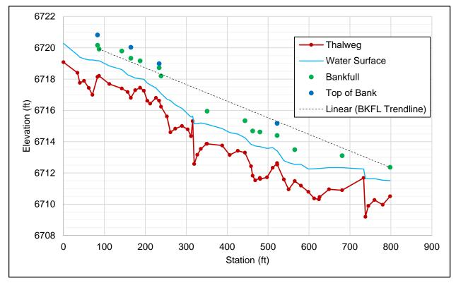
Figure 11. Longitudinal profile through Upstream Reference Reach.
