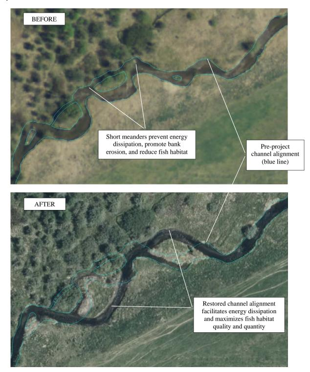
Figure 115. An unstable channel alignment (top) was corrected through construction of suitable meander pattern (bottom). The constructed meander pattern maintains aquatic habitat complexity associated with riffles and lateral scour pool bed features to maximize fish habitat.
