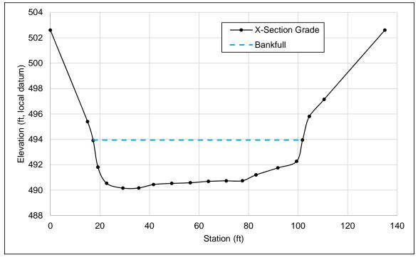
Figure 86. Typical riffle cross section in the Bullion Bridge Reach.
