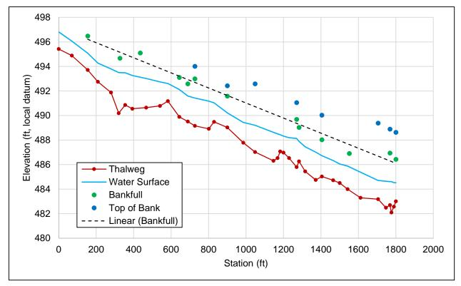
Figure 50. Longitudinal profile through the Ski Hill Reach.
