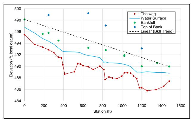
Figure 100. Longitudinal profile through Broadford Reach
