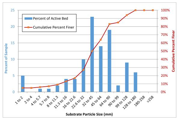
Figure 35. Surface particle size class distribution in the Training Channel reach.
