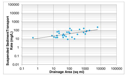
Figure 7. Suspended sediment transport rate regional curve.
