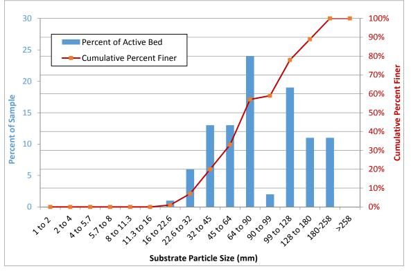
Figure 81. Surface particle size class distribution in the Downstream of Deer Creek Reach.
