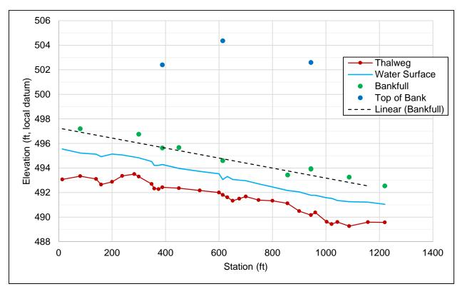
Figure 85. Longitudinal profile through the Bullion Bridge Reach.
