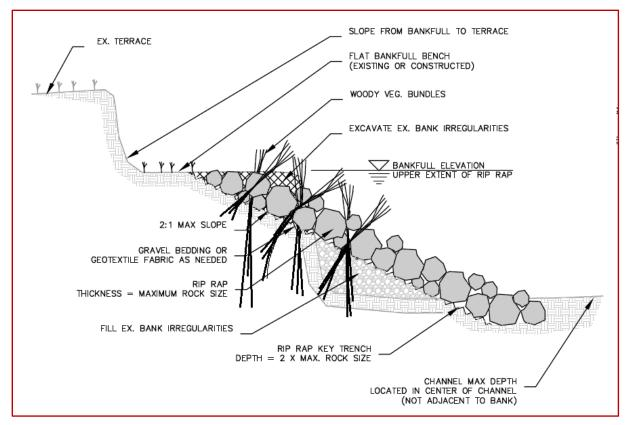
Figure 120. Profile view of typical bank rock protection treatment.
