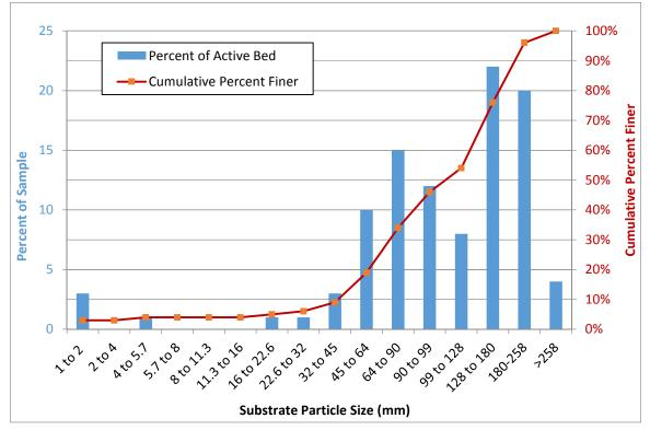
Figure 67. Surface particle size class distribution in the Highway 75 Reach.
