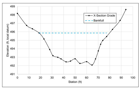
Figure 22. Typical riffle cross section in the USGS Stream Gauge Reach
