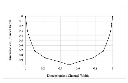
Figure 112. Dimensionless design Bc-type channel geometry, Big Wood River project area.
