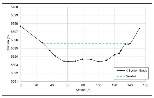
Figure 66. Typical riffle cross section in the Highway 75 Reach.
