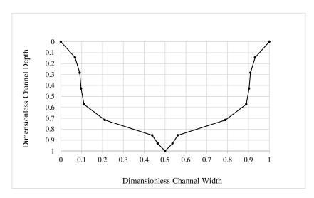
Figure 111. Dimensionless design C-type channel geometry, Big Wood River project area.
