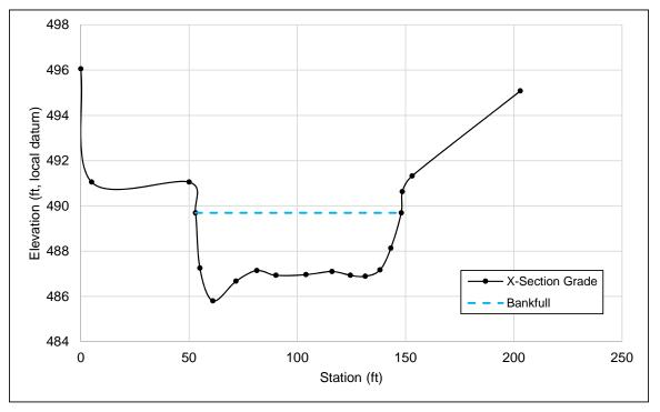
Figure 51. Typical riffle cross section in the Ski Hill Reach.
