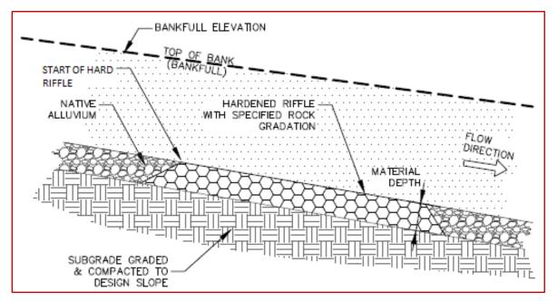
Figure 127. Profile view of typical hardened riffle treatment design.
