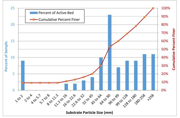
Figure 13. Surface particle size class distribution in the Upstream Reference reach.
