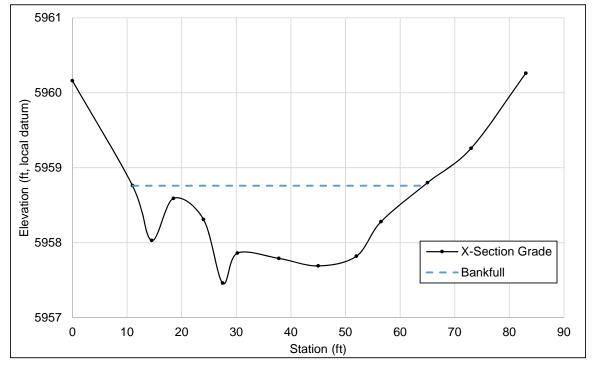
Figure 33. Typical constructed sill cross section in the Training Channel Reach.
