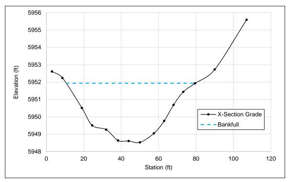
Figure 34. Typical riffle cross section in Training Channel Reach.
