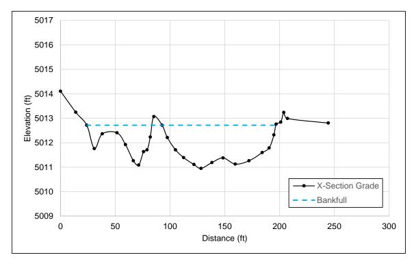
Figure 108. Typical riffle cross section in the Glendale Reach.
