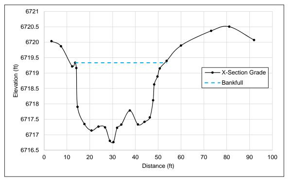
Figure 12. Typical C-type riffle cross section in Upstream Reference Reach.
