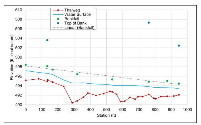
Figure 71. Longitudinal profile through the Downstream of East Fork Reach.
