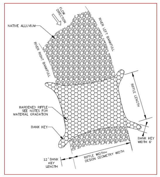
Figure 128. Plan view of typical hardened riffle treatment design.
