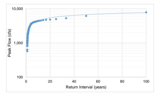
Figure 2. Peak flow recurrence interval at the USGS Big Wood River gauge at Hailey (#13139510).
