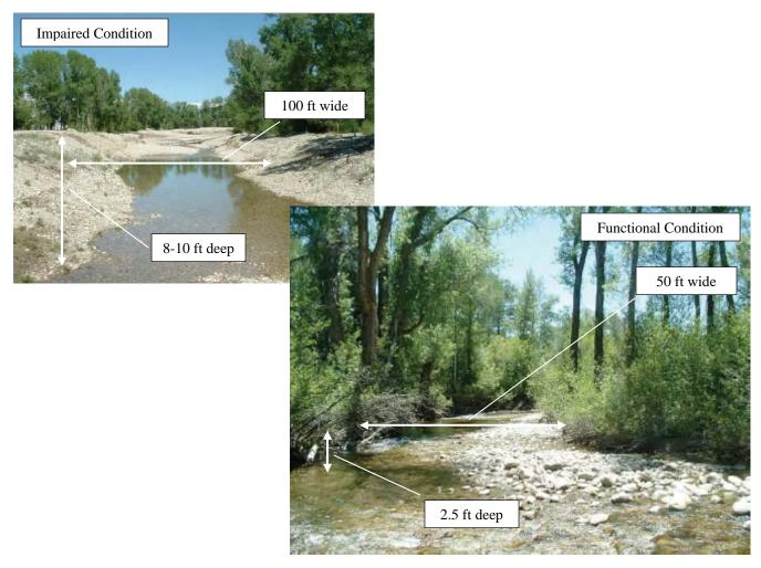
Figure 114. The over-widened and degraded river channel (top) was narrowed and shaped to mimic stable functional conditions (bottom). The functional channel with proper width, depth, profile, and alignment (bottom) provides river functions and fish habitat superior to those of the impaired channel condition (top).
