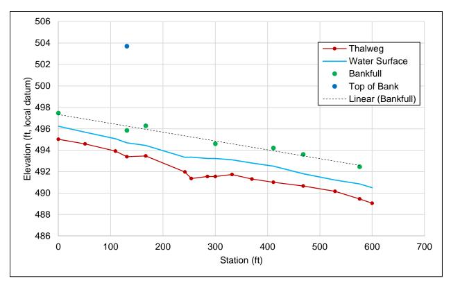
Figure 17. Longitudinal profile through Wood River Campground Reach.
