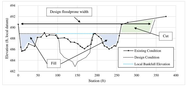
Figure 123. Typical existing and design floodplain geometry.
