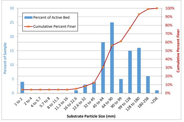
Figure 87. Surface particle size class distribution in the Bullion Bridge Reach.
