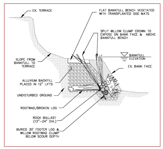
Figure 116. Profile view of typical wood revetment bank stabilization treatment.
