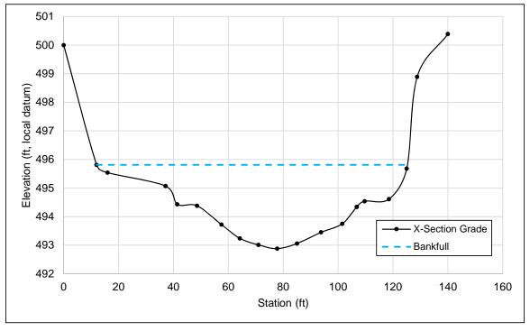
Figure 101. Typical riffle cross section of main channel in Broadford Reach.
