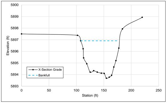
Figure 42. Typical riffle cross section in the Hulen Meadows Reach
