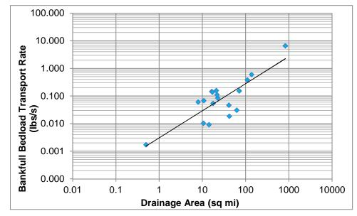
Figure 6. Bedload sediment transport rate regional curve.
