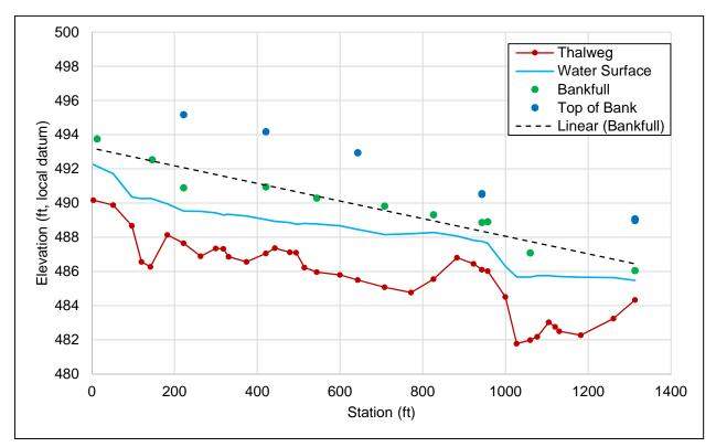
Figure 79. Longitudinal profile through Downstream of Deer Creek Reach.
