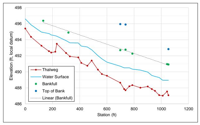
Figure 26. Longitudinal profile through Fox Creek Reference Reach.
