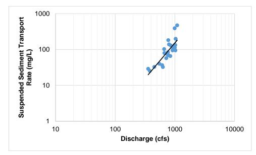
Figure 5. Suspended sediment transport rating curve, North Fork Campground on the Big Wood River.
