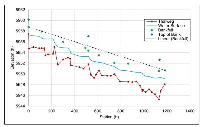
Figure 32. Longitudinal profile through Training Channel Reach.
