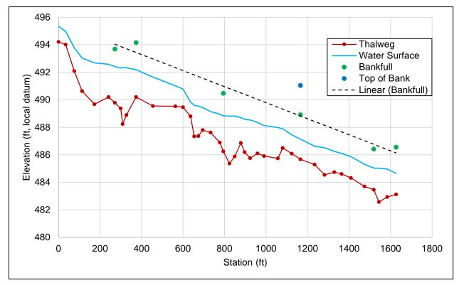
Figure 92. Longitudinal profile through the Colorado Gulch Reach.
