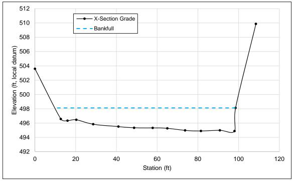
Figure 72. Typical riffle cross section in the Downstream of East Fork Reach.
