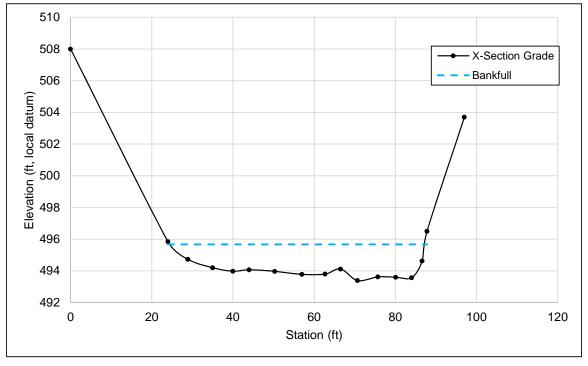
Figure 18. Typical riffle cross section in Wood River Campground Reach.
