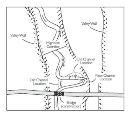
Schematic of a channel within a channel migration corridor taken from ISPG (2003). Assuming there were no bridge or other risks, no action may be an appropriate approach on a bank erosion site for a channel completely within its migration corridor that does not threaten public safety or infrastructure.
