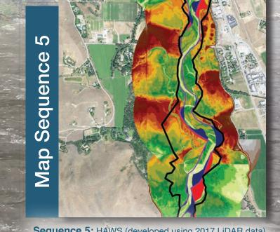
Sequence 5: HAWS (developed using 2017 LiDAR data) mapping with areas of recent channel migration in blue and high erosion potential areas in red
