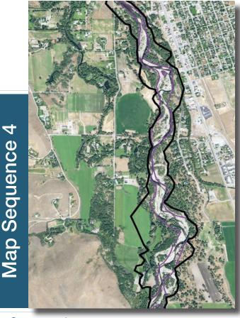
Sequence 4: 2015 Aerial Photo with the 2017 channel boundary in purple and the HCMZ in black. The areas in between are considered Zones of Moderate Erosion Potential.
