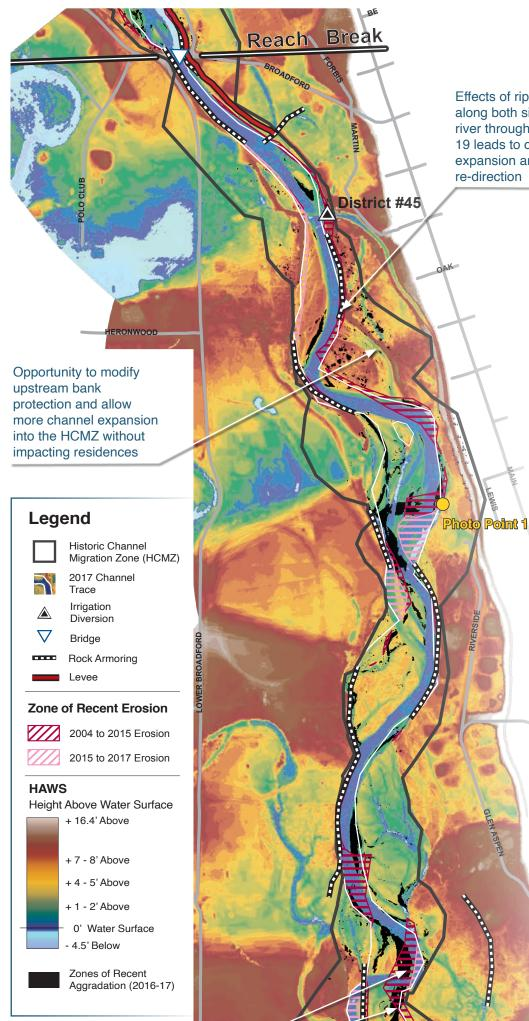
Effects of riprap along both sides of river through Reach 19 leads to channel expansion and flow re-direction
