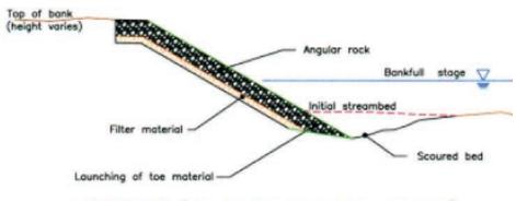
LAUNCHED TOE (after toe has launched into scour hole)
