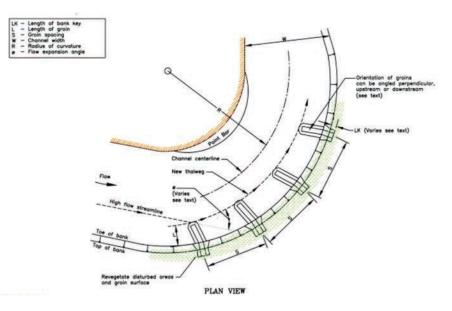
Conceptual layout of groin field taken from ISPG (2003). In place of riprap rap groins, a more ecologically friendly option is to utilize ELJs (large wood groins) in place of riprap; Courtesy of Cardno.
