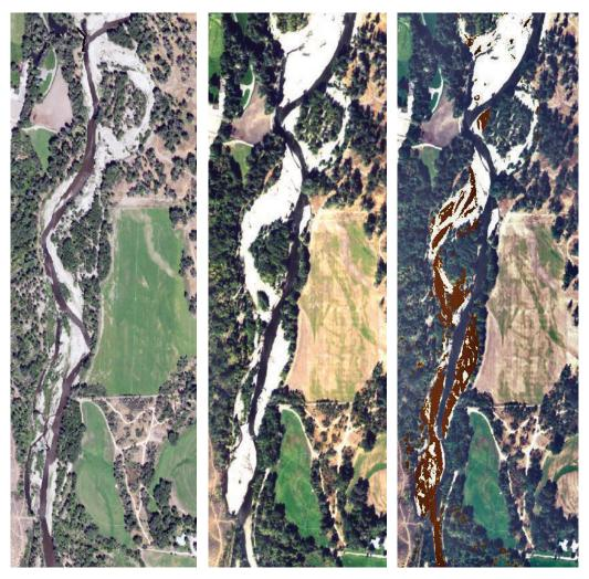
Areas of sediment deposition; 2015 image on left; 2017 image in center; and, sediment deposition from 2017 flood shown in brown over the 2017 aerial photo, image on right.
