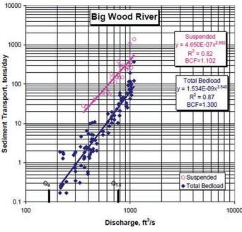
• Above: Schumm's classic figure: Channel classification based on pattern and type of sediment load, showing types of channels, their relative stability, and associated variables (After Schumm 1981). The Big Wood River sediment load has a high percentage of bed load (>11%) versus total load, as measured by the USFS (see accompanying image to the left), indicating relatively low inherent channel stability.
