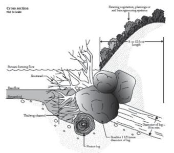
Log rootwad and boulder revetment; Courtesy of Cardno.
