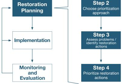
**Diagram of the river restoration process;** four steps for identifying and prioritizing river restoration actions that are nested within this [hierarchical strategy] broader process. Beechie et al (2008).
