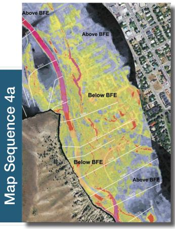
Sequence 4a: Relative Elevation Model (REM) and BFE
