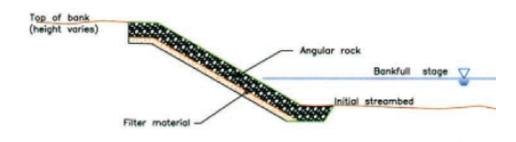
LAUNCHABLE TOE (Before toe is launched into scour hole)
