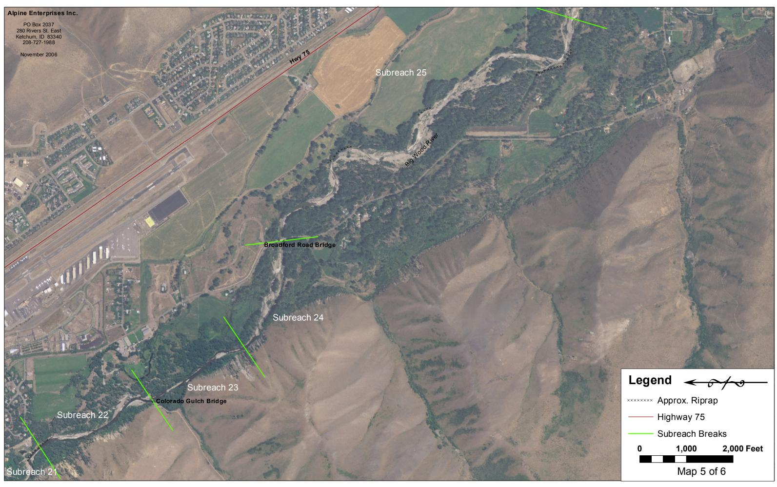
Figure 5 (Sheet 5 of 6). Results of the preliminary bank hardening survey for the Big Wood River within the study reach.
