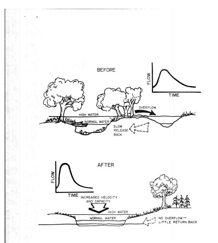
Fig. 15. Comparison of off-channel storage and return of flood water before and after channelization (Simpson et al. 1982).
