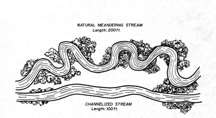
Fig. 16. Effect of channelization on stream length.
