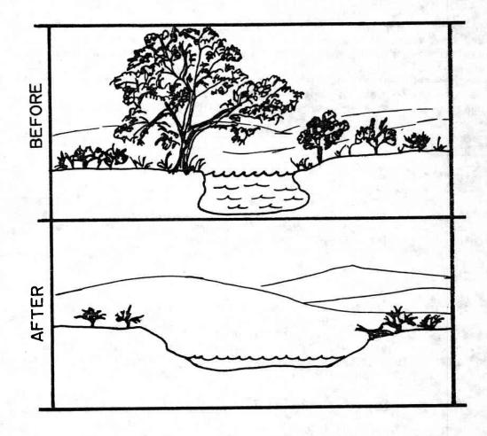
Fig. 12. Changes in cross-sectional channel profile due to riparian degradation.
